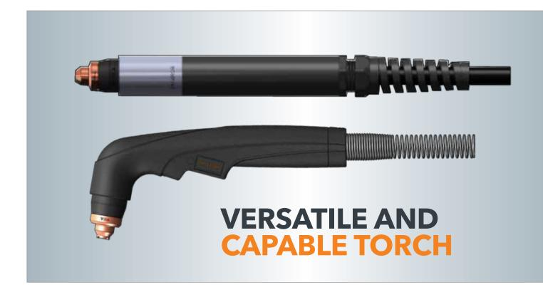
The lightweight FHT-EX®40H hand and machine torches with flexible cables are suitable for a wide range of applications and ideal for mobile use. These torches are optimally designed for use with EX-TRAFIRE<sup>®</sup>40SD power sources and are suitable for cutting and grid-cutting. They provide precise cutting results on plate thicknesses of up to 15 mm and more.
